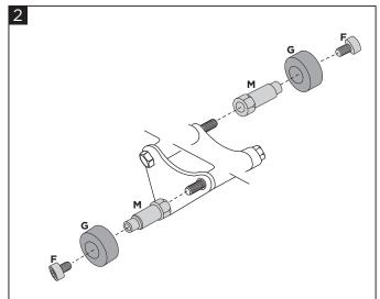
Take off the original sell locking nuts and tighten the bearings (M), with the grommets (G) and the screws (D).
